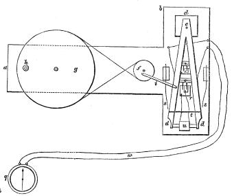
copper rod connecting the two arms of the lever to give strength; u the hollow helix fixed, or moveable at pleasure. The plan is to a scale of one-fifteenth. Being on a
